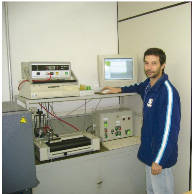
Mr. Emerson Paredes from Mahle Metal Leve inspecting piston pins with Rollscan 200 system.
