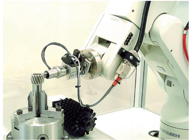
RoboScan takes care of the gear inspection after the gear has been manually placed on the stand.
