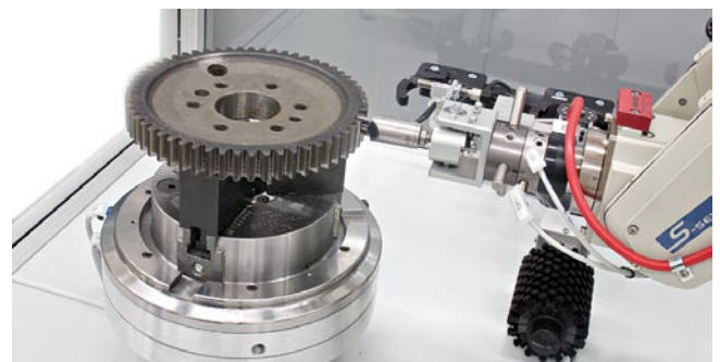
Rollscan 250 sensor installed in the RoboScan and measuring a gear.
